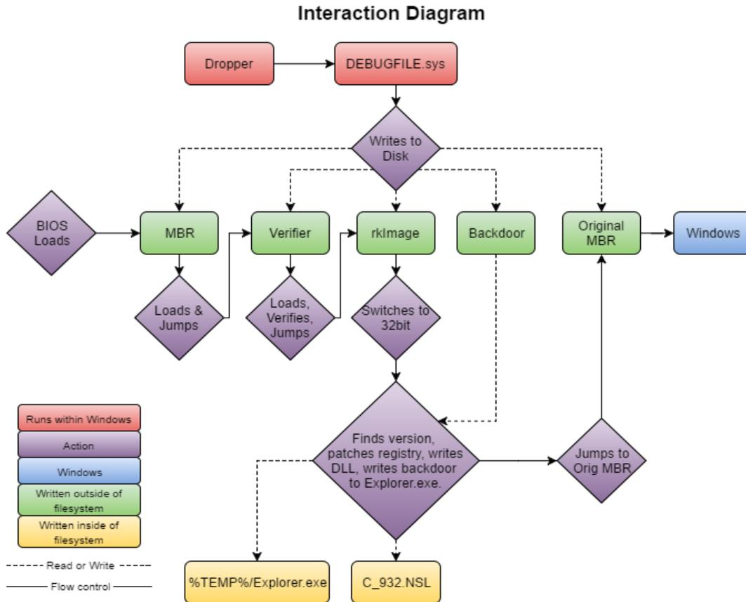
Figure 9: Diagram showing the out-of-OS boot process.
