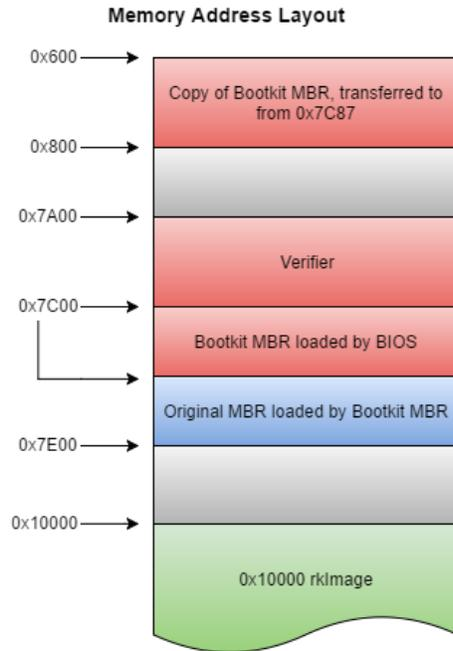
Figure 7: Address layout of memory loaded before rkImage
